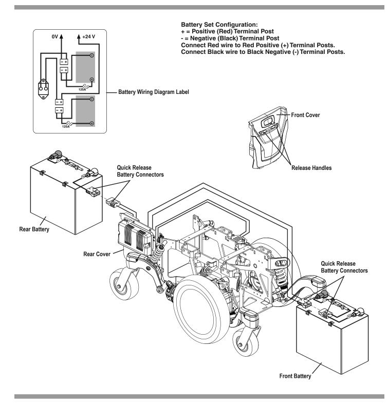
Figure 14. Battery Installation
