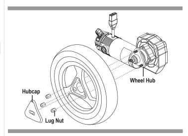
Figure 12. Drive Wheel with Three Lug Nuts and Hubcap
