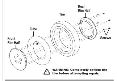
Figure 13. Drive Wheel Disassembled
