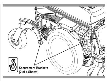
Figure 6. Transit System Securement Brackets
