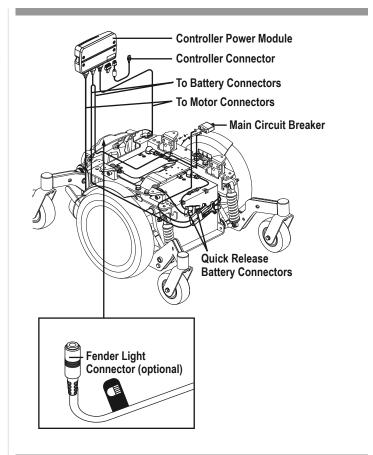
**Figure 1. Electrical Components**
