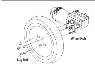
Figure 11. Drive Wheel with Five Lug Nuts
