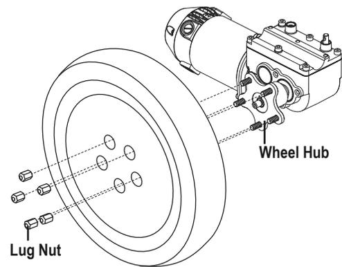
Figure 11. Drive Wheel with Five Lug Nuts
