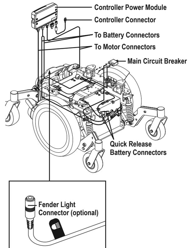
**Figure 1. Electrical Components**
