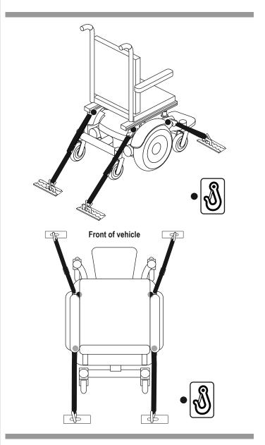
Figure 7. Unoccupied Transit System Securement Points
