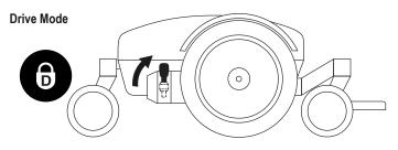
Figure 2. Manual Freewheel Lever Operation
