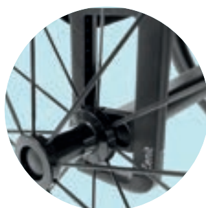
Drive wheel adapter, permanently welded
