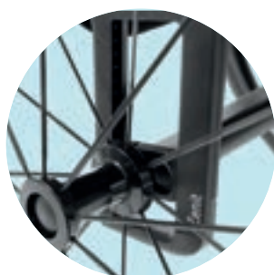
Drive wheel adapter, per- manently welded
