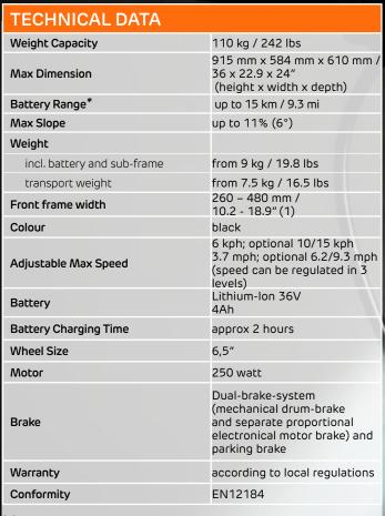
(1) Frame width measured from the center of the frame tube to the center of the frame tube at mounting position.
